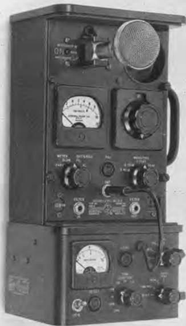
Figure 4. View of Impact Noise Analyzer attached to a sound-level meter.
